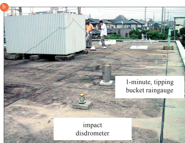
8 (a) 2D-video disdrometer placed on the rooftop of the NIED Hiratsuka Testing Yard (Hiratsuka, Kanagawa). (b) One-minute interval data recording tipping bucket raingauge and impact disdrometer placed at the same location.
